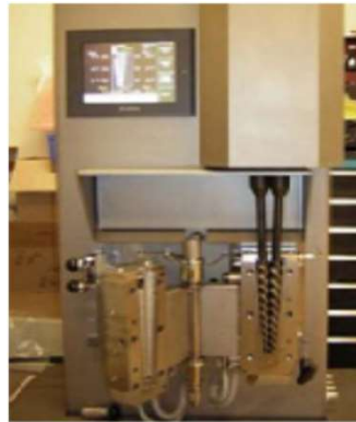
Twin- screw extruder
