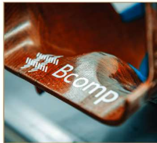
Thanks to the powerRibs™ technology, it is the first time that natural fibre composites can replace carbon fibres. ©McLaren
